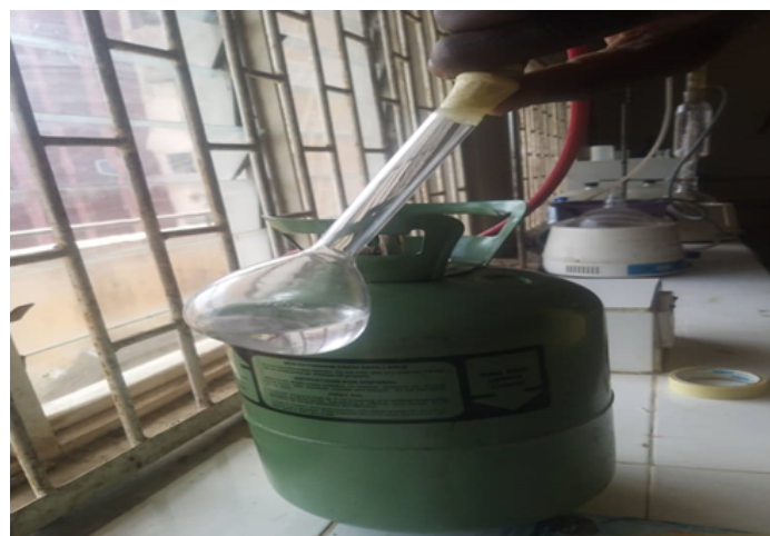
Fig. 5. Newly prepared sodalime solution (CaHNaO 2 ) before CO 2 gas reaction.
