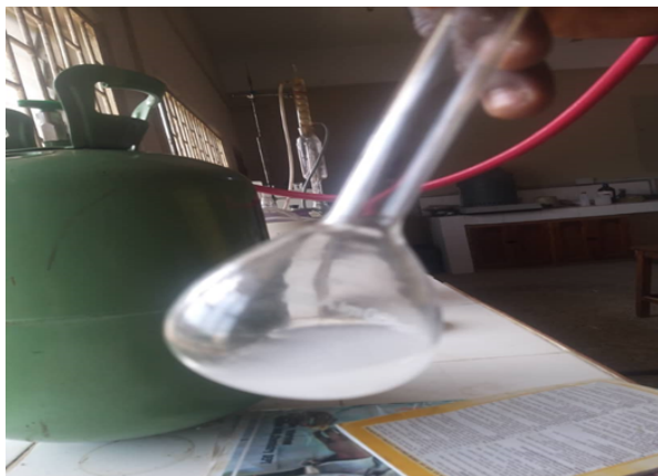
Fig. 6. Sodalime solution ( \text{CaHNaO}_2 ) turned milky after reaction with \text{CO}_2 gas.
