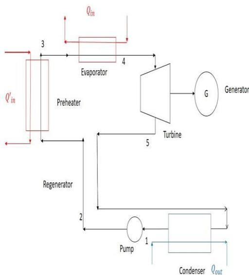
Fig 1. Schematic Diagram for Rankine cycle
