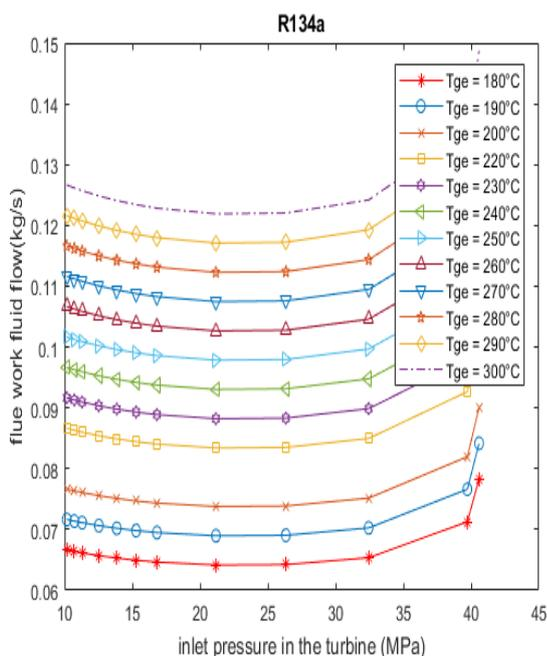
Fig. 3. Work fluid flow for a fixed flue gas temperature (R134a)
