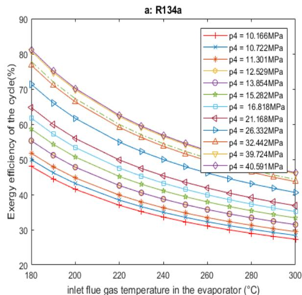
Fig. 60 Exergetic efficiency in function of flue gas inlet temperature
