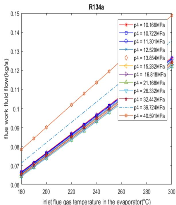
Fig. 4. Work fluid flow for a fixed flue gas pressure (R134a)
