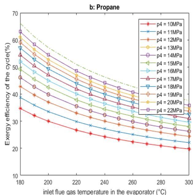
Fig. 71. Exergetic efficiency in function of inlet flue gas temperature
