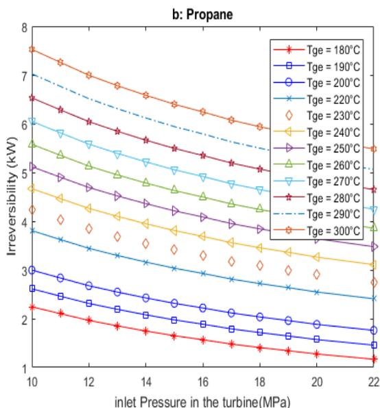
Fig. 13. Irreversibility in the evaporator in function of turbine inlet pressure
