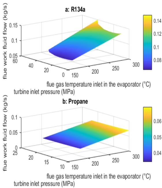
Fig. 5. Work fluid flow in function of inlet turbine pressure and inlet gas temperature
