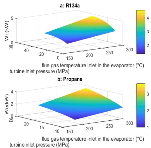
Fig. 6. Electric power in function of turbine pressure inlet and flue gas temperature inlet
