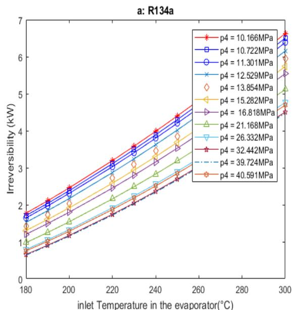
Fig. 95. Irreversibility in the evaporator in function of flue gas inlet temperature
