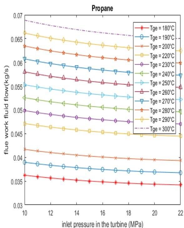
Fig. 2. Work fluid flow for a fixed flue gas temperature (Propane)
