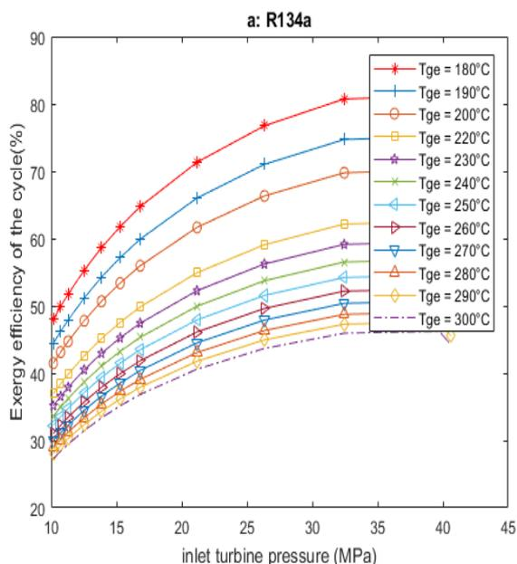
Fig. 82. Exergetic efficiency in function of turbine inlet pressure
