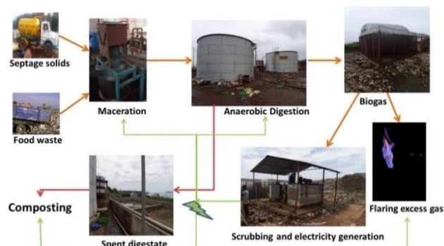
Fig. 2. Process flowchart of full-scale biogas plant at Vasco, Goa.
