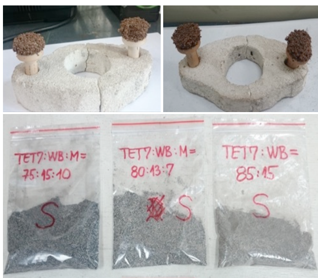
Fig. 8. Samples of deposits and slag during co-firing of lignite with different types and content of biomass in the mixture - see also [26] and [29].
